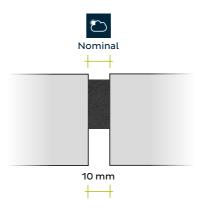
... in the summer period, see the drawing below, the **B. Determine the correct tape depth** adjacent building elements will elongate due to heat absorption. The joint will compress from 10 till 8 mm. The BOSTIK M600 TAPE'N'TIGHT BG1 15/5-10 could still be the preferred dimension to apply, however...
