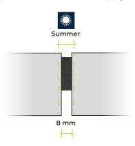
... in the winter period the adjacent building elements will decrease in length due to colder temperatures. The joint will expand from 10 till 12 mm. The **BOSTIK** M600 TAPE'N'TIGHT BG1 15/5-10 cannot perform properly. UV-stability and rain resistance will cause problems.
